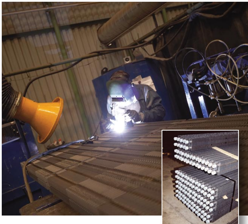
The gilled tube design is used in our large capacity MISSION™ XW-TG exhaust gas boilers/economizers as well as in the standard MISSION™ XW design of boilers after diesel engines. The spacing of the gilled tubes is calculated to minimize soot build-up. Cleaning with water washing or soot blowing keeps the EGB efficient.
