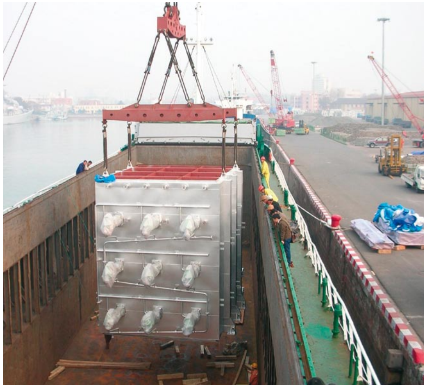
The gilled tube design is used in our large capacity MISSION™ XW-TG exhaust gas boilers/economizers as well as in the standard MISSION™ XW design of boilers after diesel engines. The spacing of the gilled tubes is calculated to minimize soot build-up. Cleaning with water washing or soot blowing keeps the EGB efficient.
