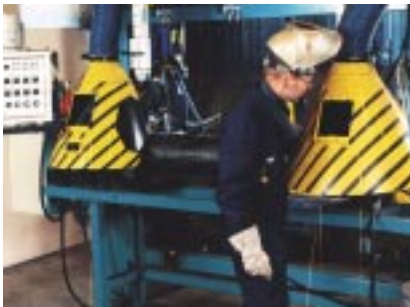
Pin tube welding
